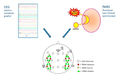
*Fig. 1: Simultaneous assessment of electrophysiological and vascular signals by means of the electroencephalography and the functional near-infrared spectroscopy.*
