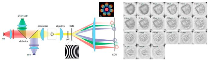
Fig. 2: Synthetic Holographic Microscopy: Multi-plane imaging by wavefront shaping with a spatial light modulator. Using RGB illumination and a colour camera, 21 planes of the sample (a spore) could be imaged simultaneously (A. Jesacher et al., Optics Express, 21, 11150, 2013).
