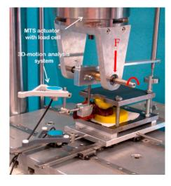
Fig. 2: In vitro test set-up used to apply physiological loading to pedicle screws and provoke screw loosening. Red arrows show the load application and the pivot axis to allow a tilting motion of the screw in the vertebral body.
